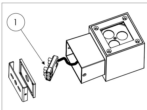
**B.** Power up the unit by using the terminal box "1".
