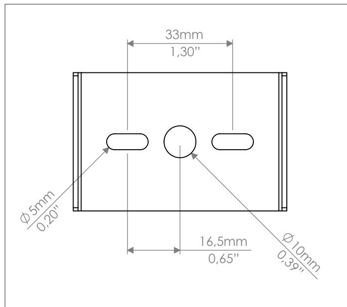
Use the two slots Ø5 to fix the fixing plate.
