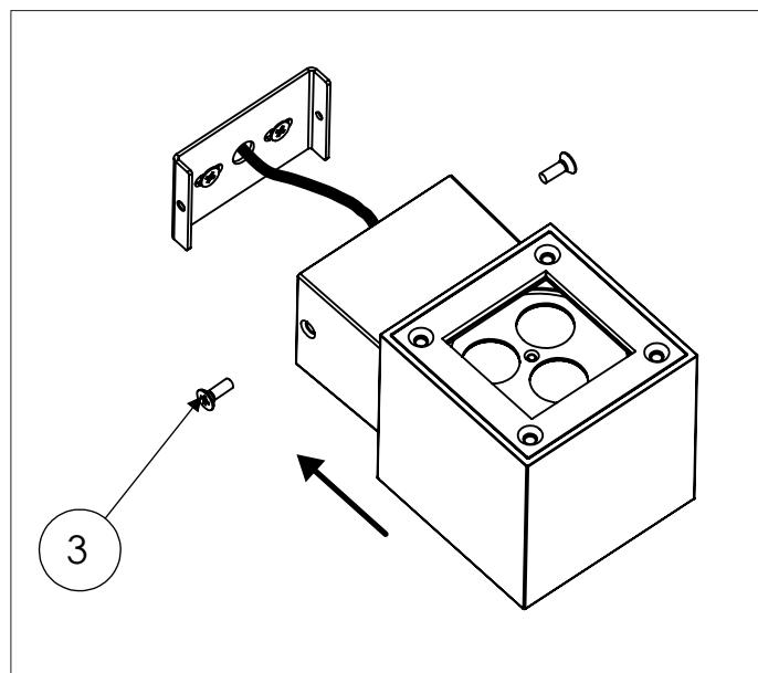
Fix the unit to the plate by using the screws "3".
