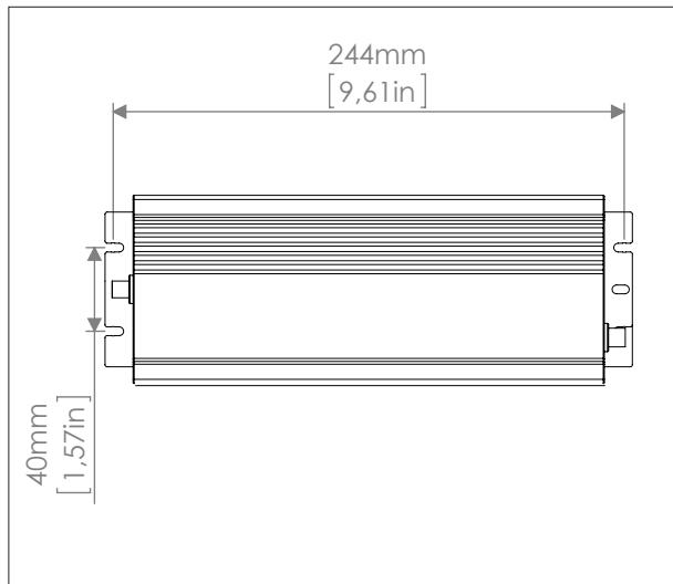
Use the four Ø4 holes (0.15") on the box in order to fix the device
