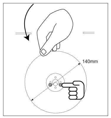
Insert the heads of the screws in the bigger slots of the new wheel.
