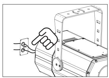
Run the cables through the holes, then fix the metal cover in place.
