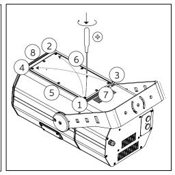
At the end of the operations, close the cover by well cross-tightening the screws.
