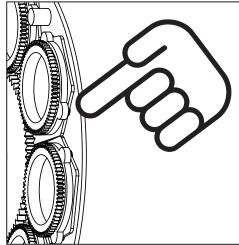
The gobo holder must perfectly fit in its slot.
