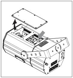
Undo the six screws to remove the cover.
