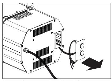
Remove the cover and pull the cables out.
