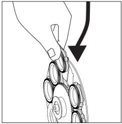
Put the new gobo in its slot, make sure that its flat side goes under the spring beneath the cog wheel.
