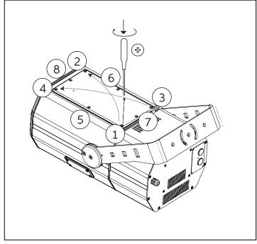
At the end of the operations, close the cover by well cross-tightening the screws.
