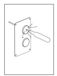
Bring the cables and pierce the two rubber seals with a screwdriver.
