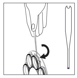
Put the tool provided along with the unit under the gobo holder as shown above.
