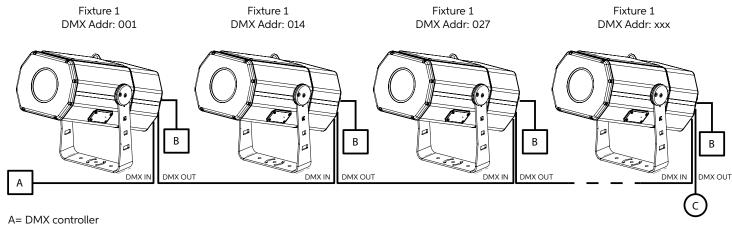
A= DMX controller B= 100-240 VAC 50/60 Hz C= 120  $\Omega$  DMX Terminator
