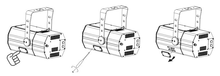
In order to access the control panel of the fixure undo the four screws as shown in the picture. After performing the operation required, close the cover by tightening the screws.
