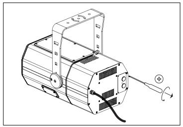
Undo the 4 screws of the metal cover.
