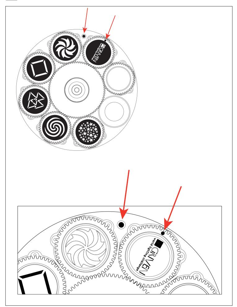
7 integrated dichroic gobos available with the interchangeable rotating gobos wheel.
