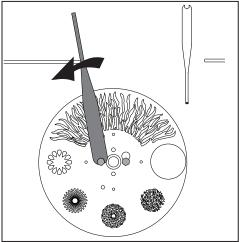
Rotate the wheel manually until it reaches the position shown above, then loosen the two screws by using the tool provided.
